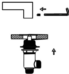
3. Place the spout in center hole of sink and handle body through right hole. (Left is red, right is blue). Assemble the rubber washer, washer and tighten with lock nut.
