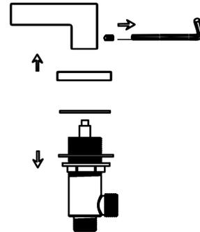
2. Remove mounting hardware from handle body. Connect water supply tube to valve body and tighten with lock nut. Do not allow the water supply brass tube to twist. Use two wrenches, as shown in the diagram, tighten the flexible hose.
