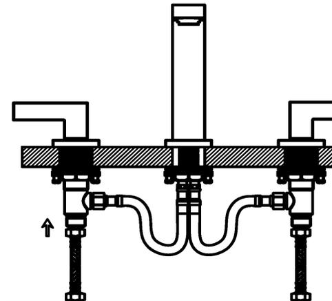
**5.** Screw and tighten the flexible hose to the faucet. Left is red, right is blue. Do not allow the water supply brass tube to twist.
